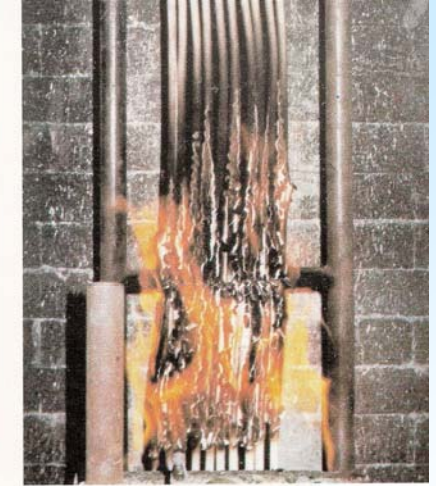
Burning cable during combustion testing
